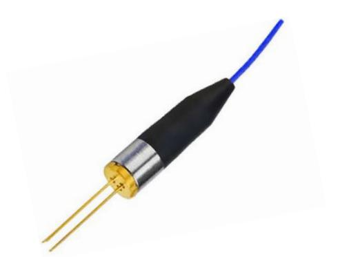
The FCML series diode lasers deliver up to 100mW of power through a 50/125 $\mu$ m fiber. They feature built-in optical isolator, low capacitance and low dark current, high stability, low threshold current, low operating current, integrated high isolation, and low insertion loss.
